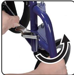
2. Unlock the buckle, then fold the pedals to the sides
