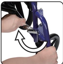
2. Rotate the foot pedal inward and lock
