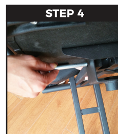
Install seat cushion using short axis (A)
